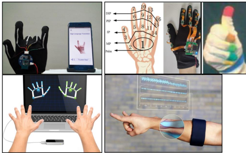
Fig 4. (a) Cyber glove, (b) data glove, (c) colour glove, (d) Leap Motion device and (e) sensors Armband.
