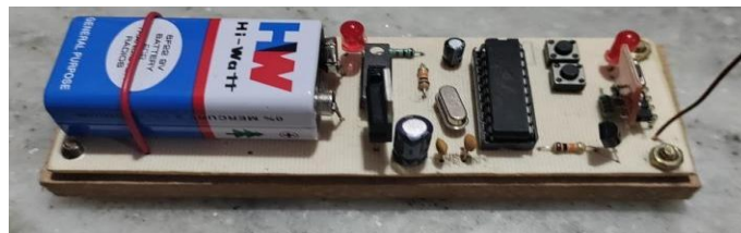
Fig 6. Circuit of RF transmitter Configuration
